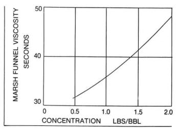
From 0.5 to 2.0 pounds per barrel (42 gals.) or 1.5 to 5.0 pounds per 100 gallons is the usual concentration of POLY-SAL for most operations. This chart is indicative of the viscosity of a well-mixed POLY-SAL fluid.
