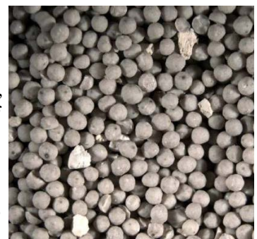
1% by weight Econo-SI5000D with 20/40 Mesh Proppant
